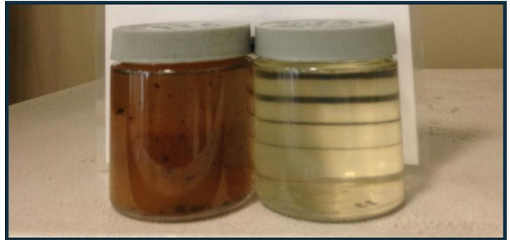
**ABOVE:** The samples pictured above contain tank samples from before (left) and after (right) the fuel restoration process took place.
