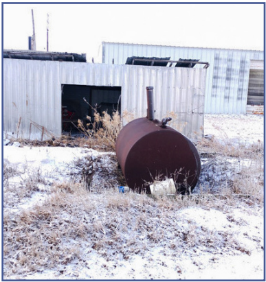
Abandoned UST tank
