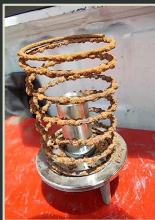
Examples of corrosion associated with ULSD.
