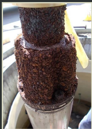
Examples of corrosion associated with ULSD.
